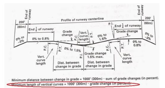
Figure 18-3b Longitudinal grade limitations for aircraft approach categories C and D. (Source: *Airport Design*, FAA Advisory Circular 150/5300-13, Changes 1–4, September 29, 1989.)
